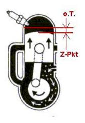
Bring the piston into ignition position. This should be 3.5-4mm BTDC.
