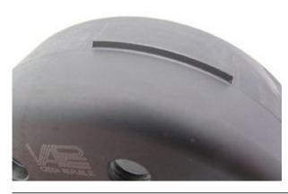
Have a look at the new rotor. You will find on its circumference a protrusion. It acts for ignition timing together with the sensor.
