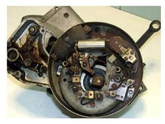
Unscrew the generator cover and take it off. Unscrew the stock dynamo and take it off.
