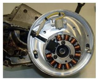
Take the cover holder plate from your new generator off. Place the preassembled unit (ground plate/stator) at the ignition seat of the crank case. Screw it down with the 2 M8 screws.
