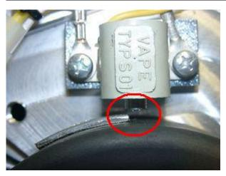
Once ignition position is achieved, take the rotor carefully off again without changing the crank position. Reset it onto the crank in such a way that the right edge of the marking on the rotor aligns with the left edge of the sensor bottom.
